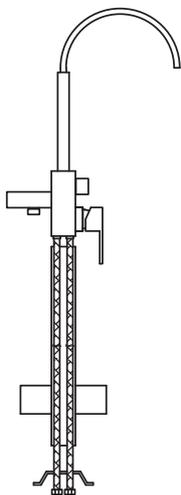
Screws the tube to body and fasten
