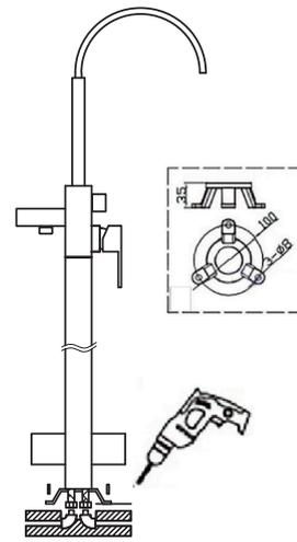
Tighten the nut and fasten
